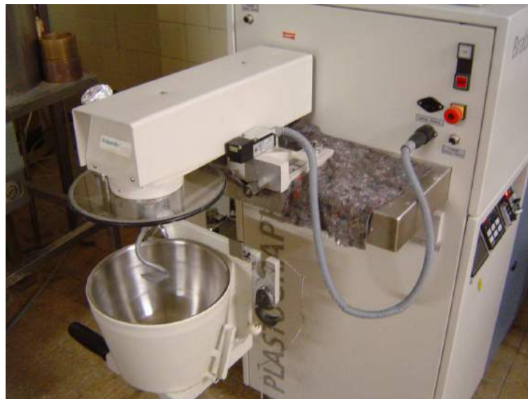
Fig. 2B.1: Picture of the planetary mixer bowl P600 investigated in connexion to the lab-station unit.
