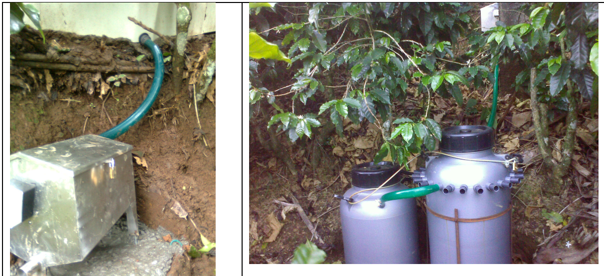
Figure 2.2. A: Runoff tipping bucket measurement equipment and B: Runoff collector containers of 40 l and 30 l capacity (right).
