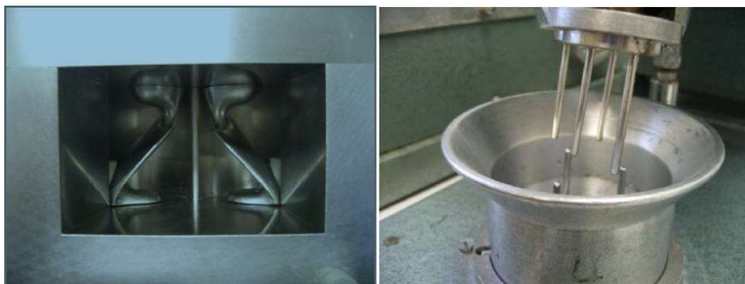
Figure 10. Geometry of the mixing system in Farinograph (left) and Mixograph (right). Copied from (Frédéric Auger, 2008)
