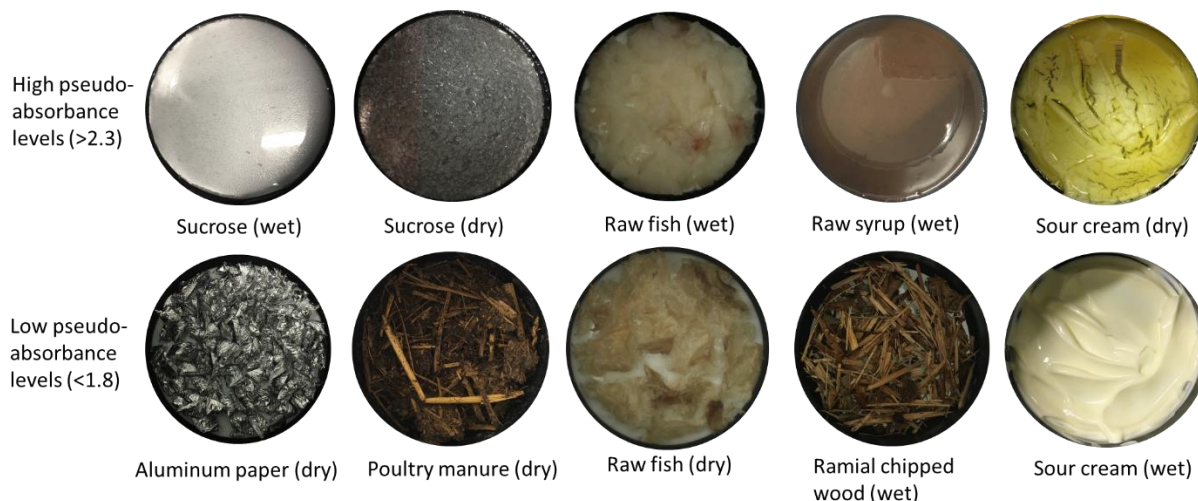
Figure 15. Visual aspect of substrates with low and high levels of pseudo-absorbance. Pictures were taken from above the NIRS measurement cell.
