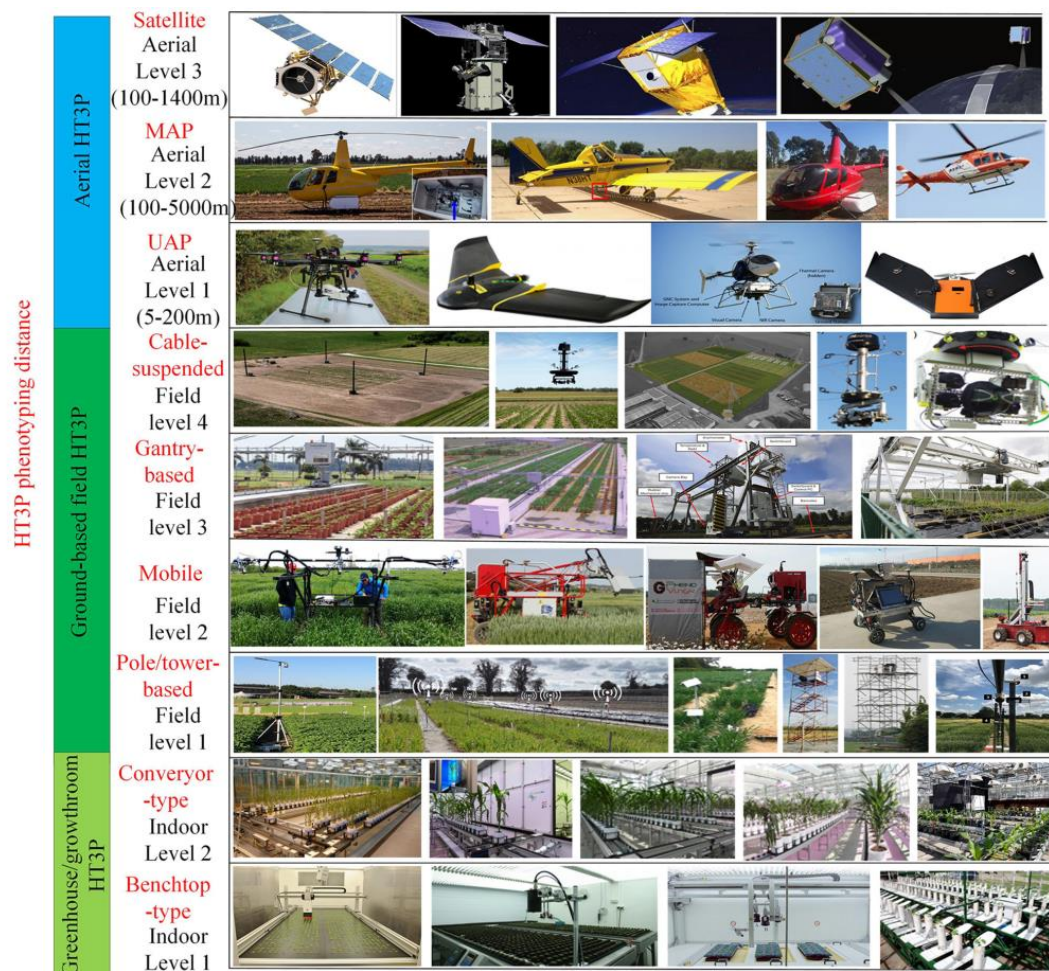
Fig. 5 : Examples of high-throughput plant phenotyping platforms (HT3Ps) as reviewed by Li et al. , (2021), including HT3Ps in the greenhouse/growth chamber, field ground-based HT3Ps and aerial HT3Ps.
